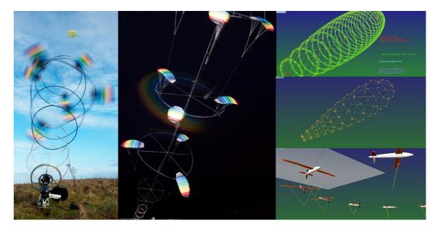
The Daisy design relies on two things. Firstly, a little lift from a lifting kite, (yellow in pictures above) this holds the turbine in the most powerful position. Secondly, Daisy needs tension in the spinning lines, to allow torque transmission. With more tension, more torque can be transmitted more efficiently. More kite layers on the stack, means more tension and therefore more power available. It's a win win.
