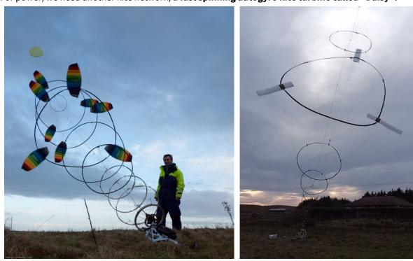
Earlier kite power research exploited line pulling and retraction (the yo-yo method) or using a kite to lift a wind turbine & send electricity down the tether (drag method) But Daisy auto-gyro kites transmit continuous torque power to ground using multiple tethers around rings as a tensioned flexible shaft. This provides better quality, constant output, with less tether drag per kite, making it more efficient.
