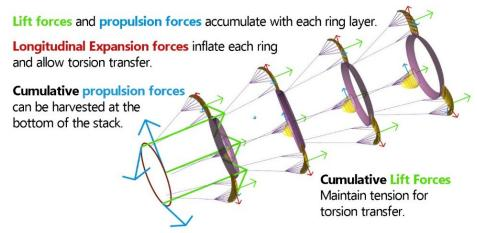
Daisy kite networks use multiple kites stacked in layers. Kite layers can be added from close to the ground all the way up a stack. Rotary kite layers help to expand the "shaft stack" which keeps powerful torque transmission viable.
