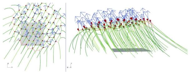
**Kites linked in a network keep their position**, despite hugely turbulent winds. Whereas individual kites on single lines, will scatter and tangle in turbulent wind, by adding a top layer of networking lines, the individual kites hold on station, even without a control system. This give a stable lifting platform.
