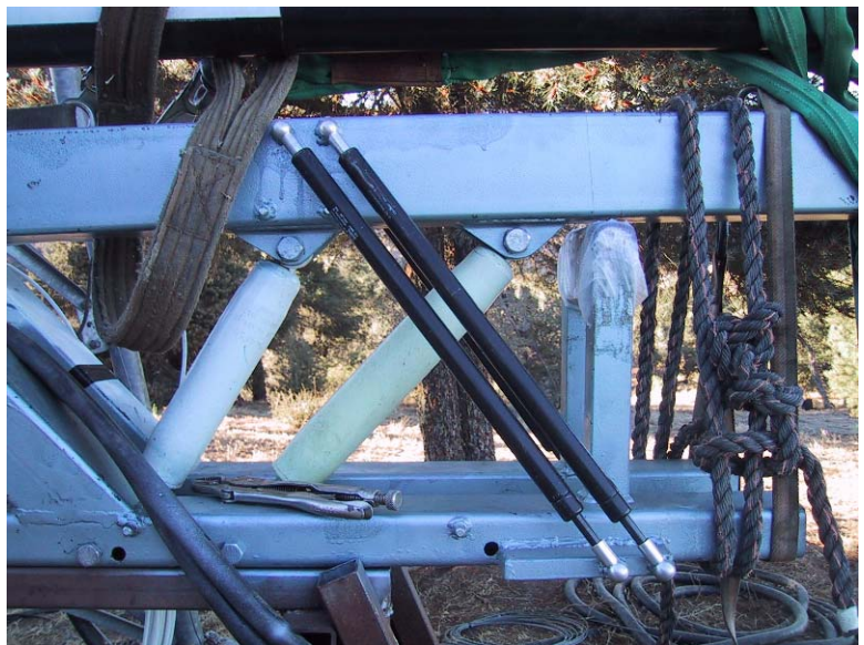
Gas shock absorbers and gas springs regulate fore-and-aft tilt for overspeed protection.
