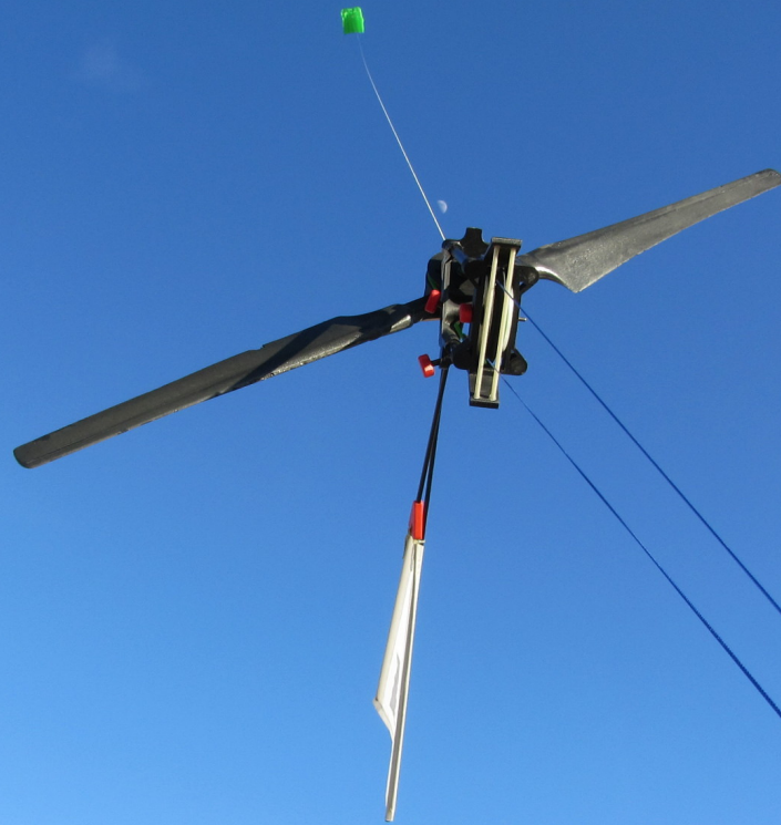
Kiwee One airborne wind turbine with 1 m rotor diameter (1 July 2017)
