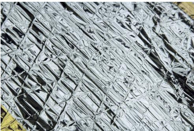
Smart – reflective coatings are reducing heat losses and temperature peaks.
