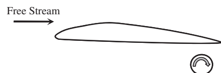
Fig. 52. Basic Vortex Flap Configuration, according to [111].
