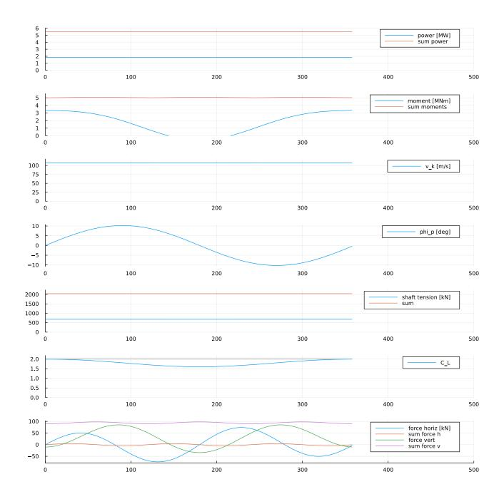
Simulation output for 12 m/s wind. The red/pink curves indicate values for all three kites, the blue/green curves for a single kite
