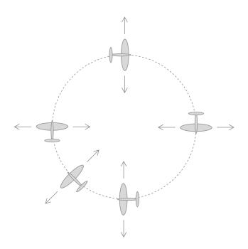
We see that we can produce such a force by rolling the kite relative to the plane of rotation. This will produce a component of lift force facing perpendicular to the path of travel. We can only produce vertical forces when we are not at the left and right sections of the looping circle. Producing vertical forces is most efficient at the top and bottom of the circle. Most of the time, we produce both a horizontal and vertical component whether we want to or not.
