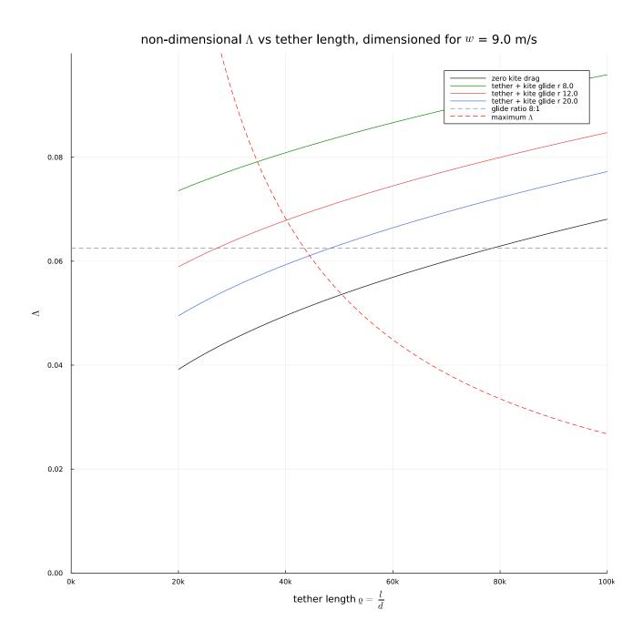
Like before, for a 8:1 overall glide ratio rig, we can read that  $\varrho$  must be around 45k or less with a kite glide ratio 20:1.
