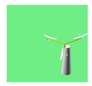
As the tethers reel out, the elevation angle is lowered gradually to let the kites face into the wind.
