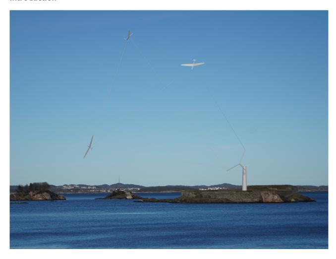
The pyramid is an airborne wind energy concept that utilizes [initially] three efficient kites in a TRPT [Torsional Rotary Power Transfer] setup. The shaft is as simple as possible with only one tether per kite and a triangular bridle at the kites.
