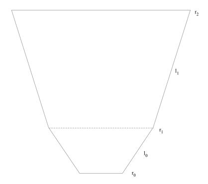
As the value of  $\Lambda$  is defined relative to the kite looping radius  $r_2$ , we need to select a matching  $\Lambda$  for the bottom shaft section.
