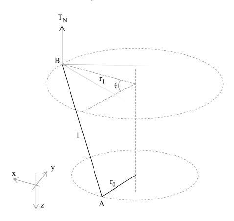
$T_N$  tether tension component normal to the plane of rotation
