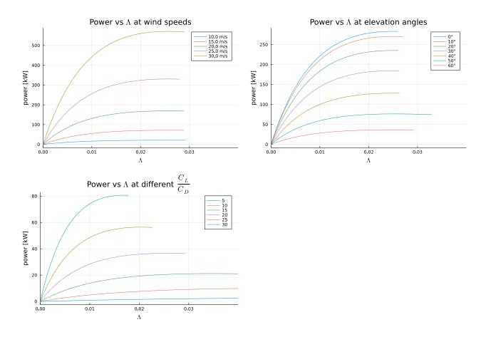
The plots are done with a nominal  $\frac{C_L}{C_D}=20$ ,  $C_L=1.5$ , wind speed 12 m/s, wing area 3 m², elevation angle 30° and  $\rho=1.225$ , unless otherwise stated.
