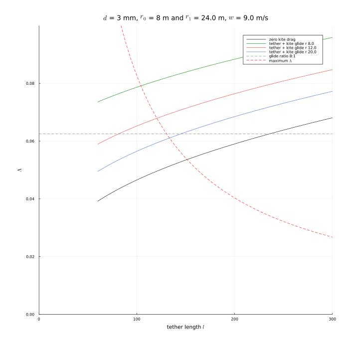
The dashed red line shows the moment-to-tension-to-radius ratio  $\Lambda$  showing the maximum amount of moment that may be transferred by a soft shaft with l of varying lengths on the x-axis. This is an absolute upper limit for that geometry. We see that if we aim for a glide ratio of 8:1 [gray dotted line], we must have a tether l shorter than 120 m approximately [where the red and gray dotted lines meet].
