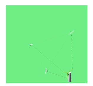
When the tethers and bridle are all fully deployed, they will rest at their end stops. The generator no longer needs to act as a motor, rather the kites drive the rotation using the power of the wind. When the kites apply their nominal high lift  $C_L$ , the generator may apply the harvesting moment. From here on, the plant may run for as long as the wind conditions are suitable.
